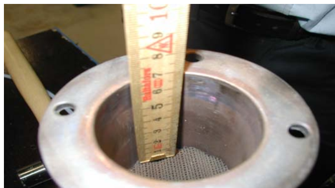
Figure 3 Corrugated metal nets with the active catalytic material (4 nets)
