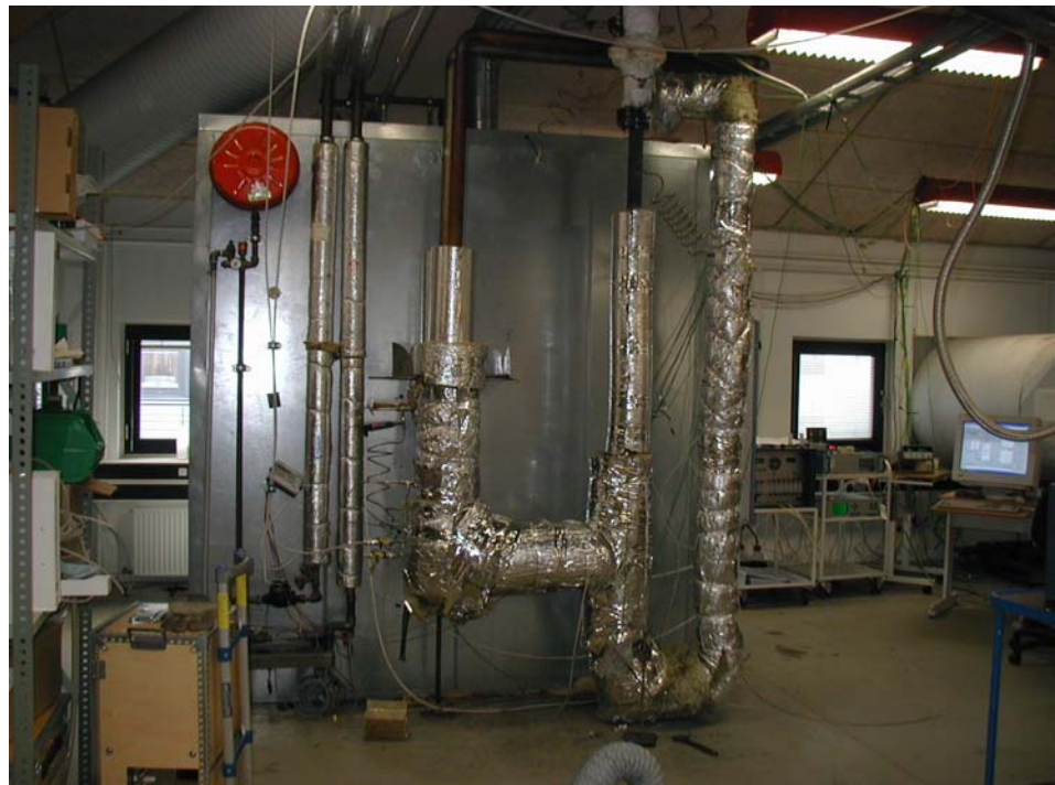
Figure 6 Picture of the test rig, the gas engine is located in the damper box
