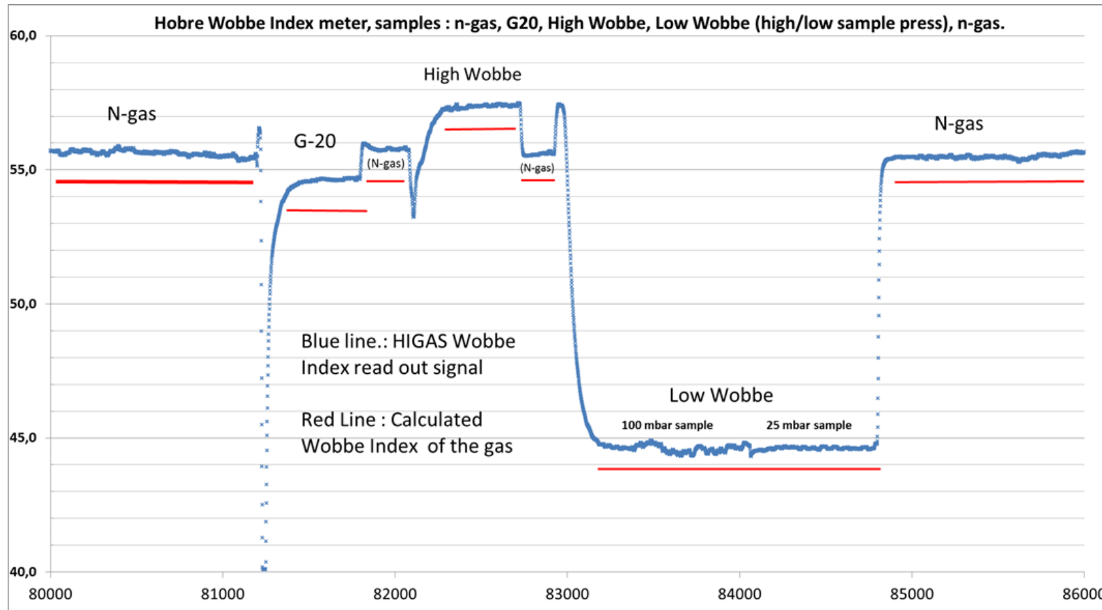
Figure 2 The DGC lab tests with the Hobré Wobbe meter. Natural gas, G-20 and two certified gas mixtures (high and low Wobbe) was used. The instrument was calibrated with G-20 at the calibration port prior to this series of measurements. When using the low-Wobbe gas, the sampling pressure was reduced from approx. 100 to 25 mbar as shown. The readout signal (Wobbe Index) was not significantly affected by this.
