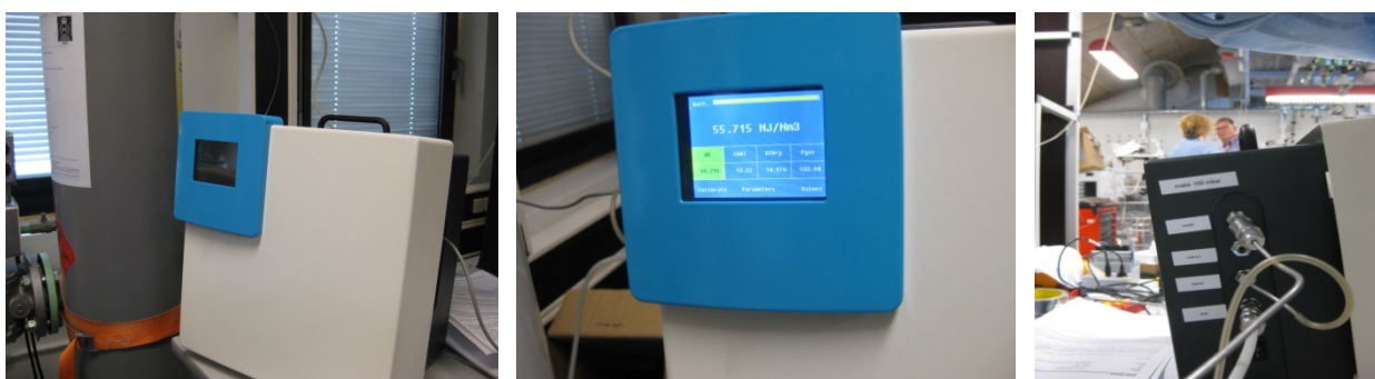
Figure 1 The Hobré Wobbe test unit, the touch display and the sample connections
