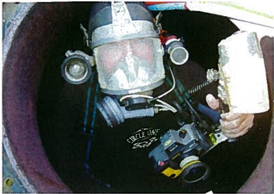
Inspection by diver in a heat storage tank. PHOTO: J.H. Dyk
