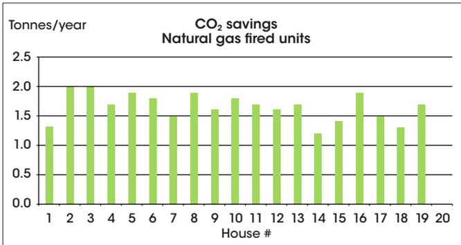
Figure 4. Carbon savings obtained in the 20 natural gas-fired micro-CHP test houses during the one-year test period. Operation in House 20 was stopped during the test period due to administrative issues in connection with the house owner's installation of solar panels at the site
