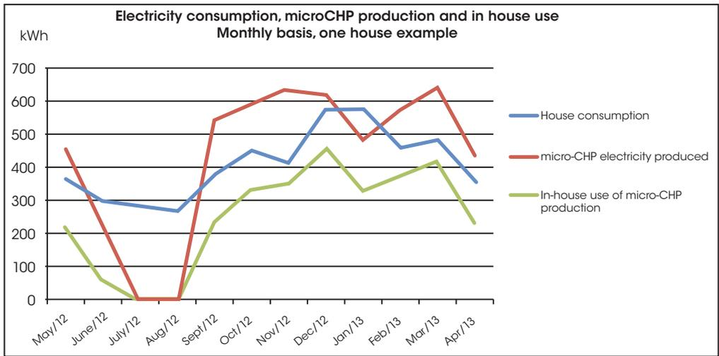
Figure 2. An example, on a monthly basis, of electricity consumption, micro-CHP production and the resulting net own use of the electricity for one test house
