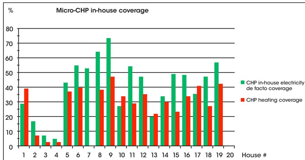
Figure 1. Micro-CHP coverage of the house's own electricity needs and the in-house heating need during the one-year test period. Houses 2, 3 and 4 are large institutions with high electricity and heat consumption, and is the reason for the low own-supply in these installations
