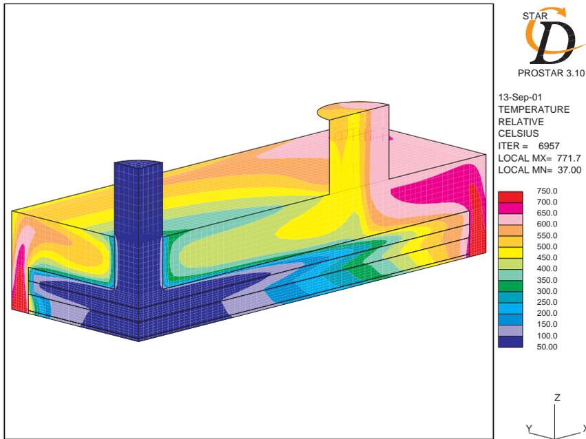
Figure 1. The calculated temperature field inside of the confined burner. ( $^{\circ}\text{C}$ )
