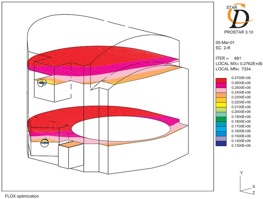
Figure 6. The calculated radiosity field in a glass furnace. ( $W/m^2$ )
