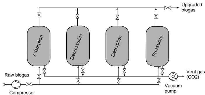
**Figure 3** Biogas upgrading system with PSA technology
