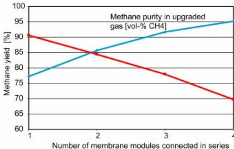
Figure 2: Relation between methane purity in upgraded gas and methane yield with membrane modules connected in series (no recycling)
