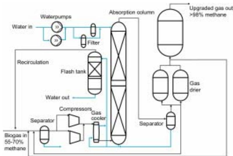
Figure 1: Removal of carbon dioxide using water wash without regeneration
