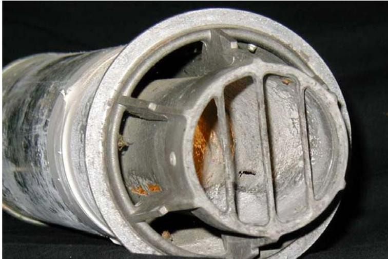
Figure 1: Example of corrosion in horizontal balanced flue
