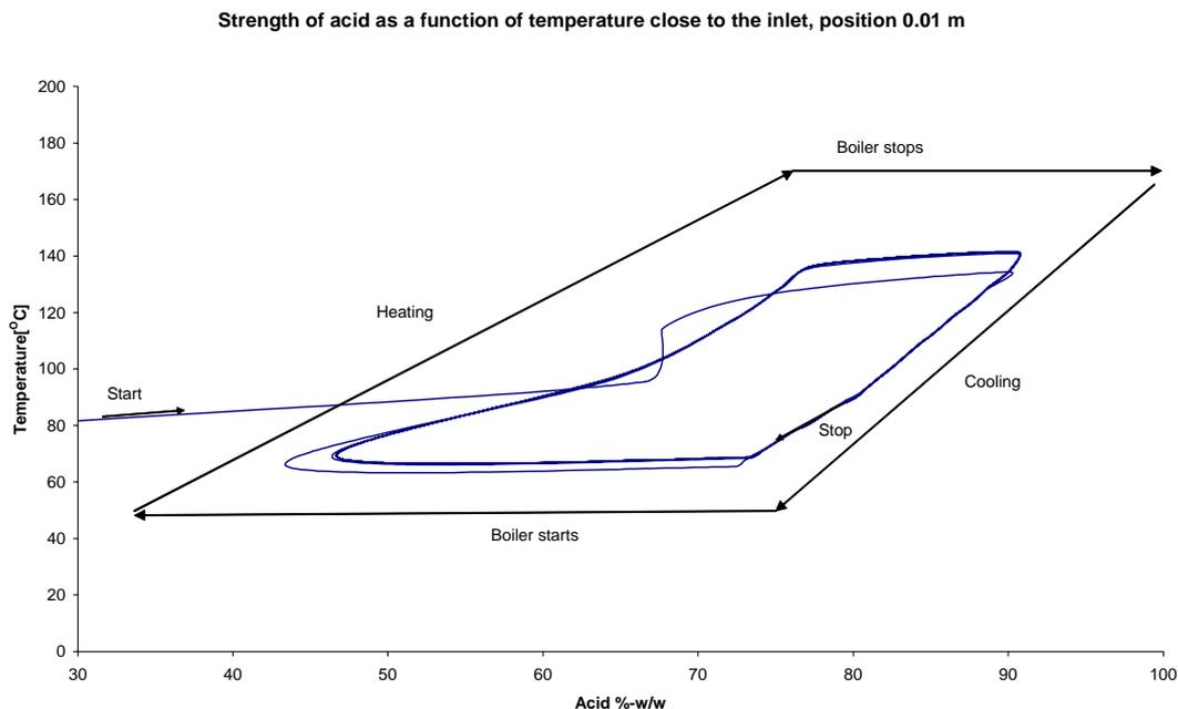
Figure 6: Mass ratio between water and acid in the acid film of a standard flue during a period of 1 hour 40 min.
