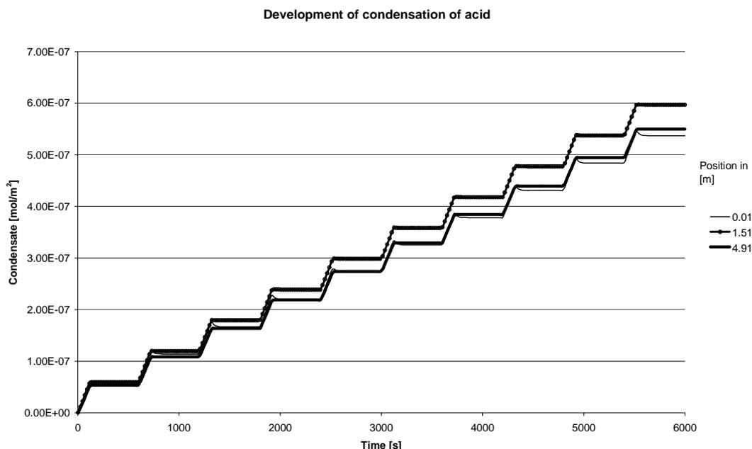
Figure 5: Total molar mass of SO<sub>3</sub> that has condensed on the aluminium surface of a standard flue during a period of 1 hour 40 min.
