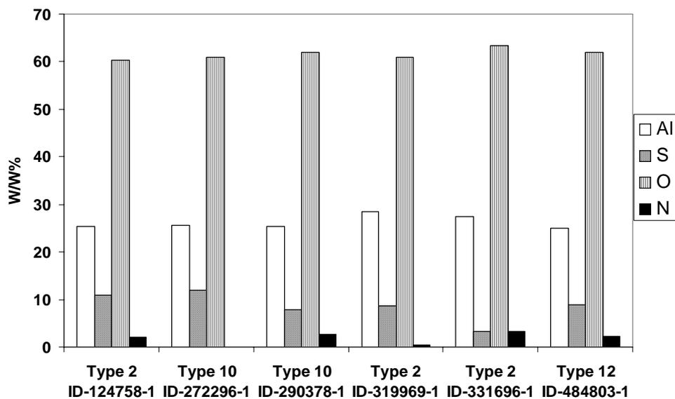
Figure 3: Analysis results for main elements. Type refers to the flue types defined.
