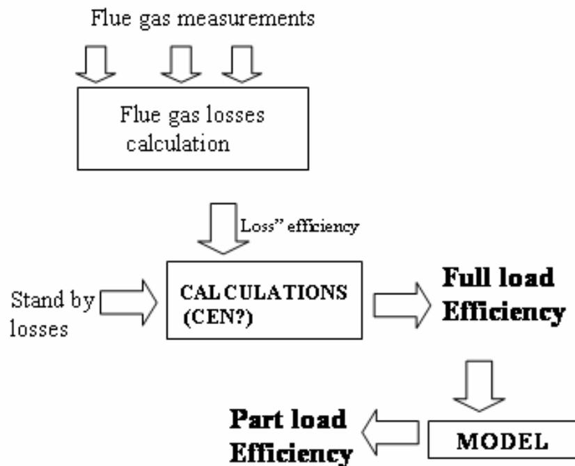
**Figure 5 Principle of the loss efficiency method**
