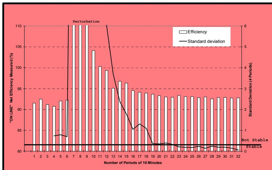
**Figure 2** Detection of stability during the efficiency test. The efficiency is measured every 10 minutes and compared with the previous values. Specific stability algorithms conclude if the thermal stability is reached and if the efficiency value measured can be validated.
