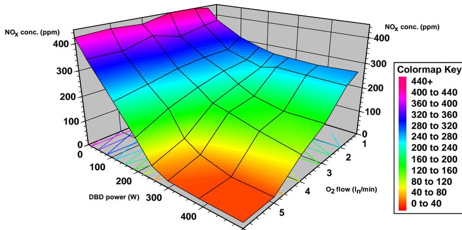
Figure 2. NO<sub>x</sub> reduction as a function of DBD effect and oxygen flow at 160 °C and with pure O<sub>2</sub> as ozone medium
