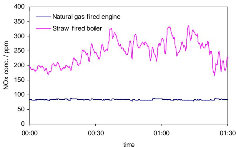
Figure 5. NO<sub>x</sub> emissions from the two plants that the deNO<sub>x</sub> unit was test on
