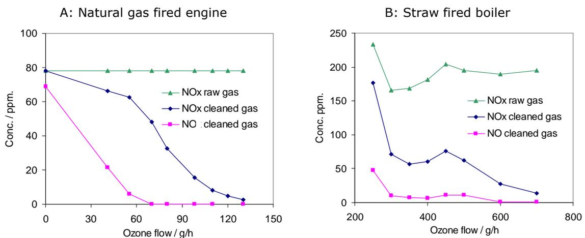
*Figure 6. Concentration of NO<sub>x</sub> in the raw flue and in the treated flue gas together with the NO concentration in the treated flue gas versus the amount of ozone supplied. Each mark for the straw fired unit represents an average value of 20 minutes of continuous measurements.*
