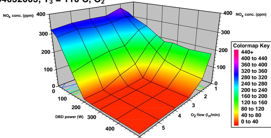
Figure 3.  $NO_x$  reduction as a function of DBD effect and oxygen flow at 110 °C and with pure  $O_2$  as ozone medium
