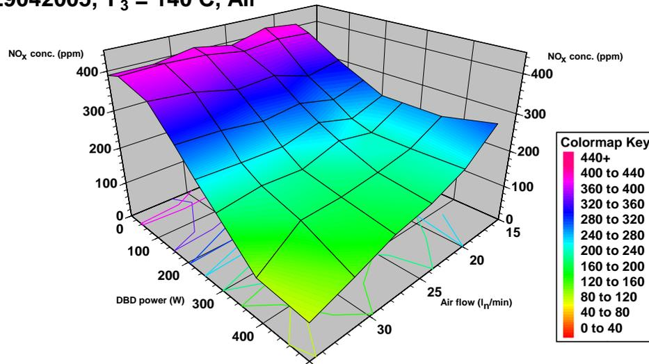
Figure 4.  $NO_x$  reduction as a function of DBD effect and oxygen flow at 140 °C and with pressurized air as ozone medium
