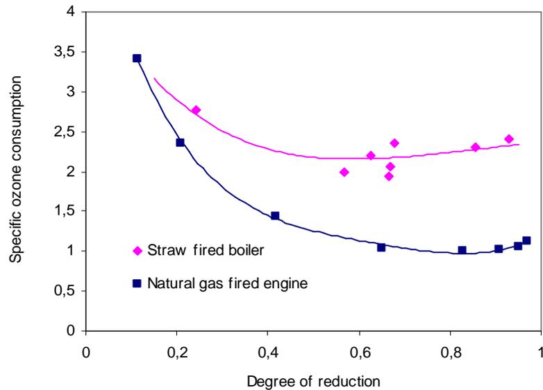
Figure 7. Specific ozone consumption versus degree of  $\text{NO}_x$  reduction. The values shown are normalised to the specific ozone consumption ( $\text{kg O}_3 / \text{kg NO}_x$  removed) for the gas engine unit at a degree of  $\text{NO}_x$  reduction of 0,8. Each mark for the straw fired unit represents an average value of 20 minutes of continuous measurements.
