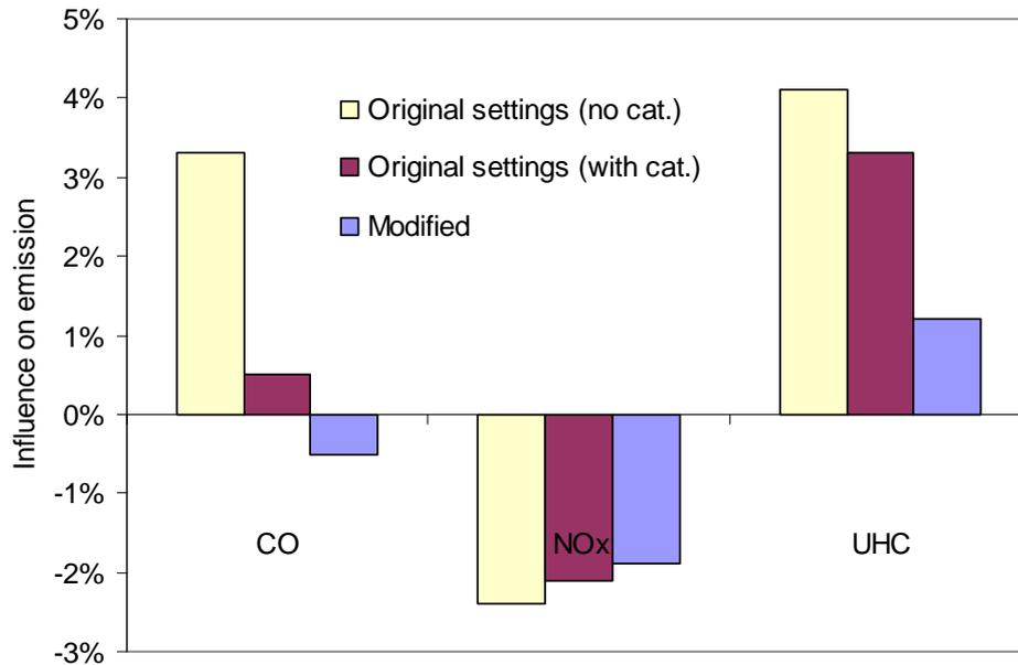
Figure 4. The influence of start and stop on the overall emissions for engine unit #4 . One warm start per 8 hours of operation compared to steady state full load operation.
