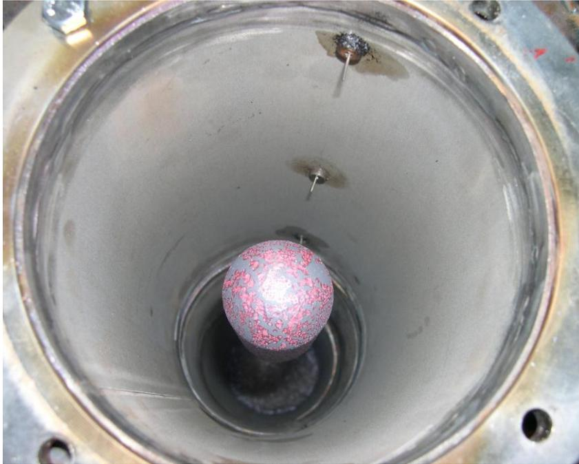
Figure 4 Cold test object in test tube
