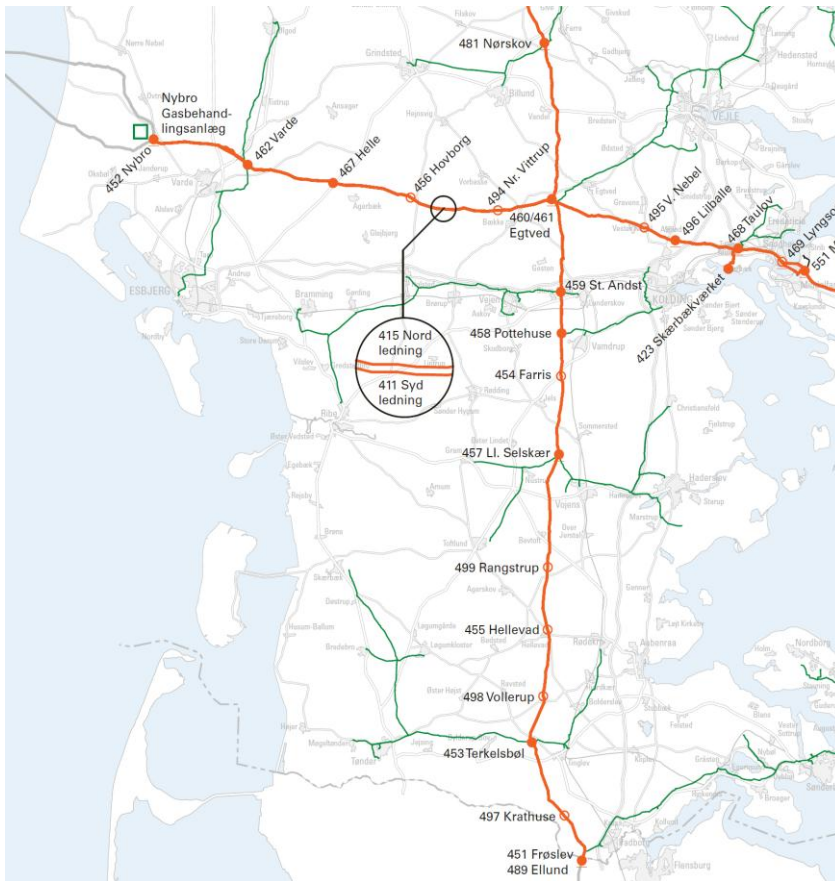
Figure 7 Detailed information points, from which data of measured or calculated actual gas composition can be found.
