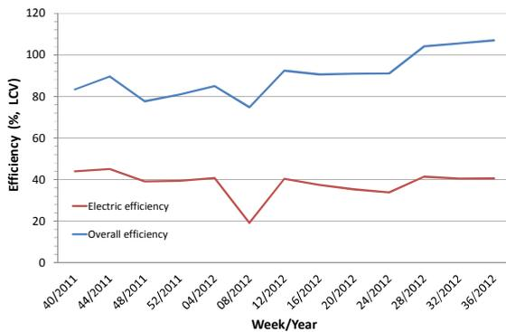
Figure 9: Hydrogen fuel cell electric efficiency from October 2011 until summer 2012 (House 18).
