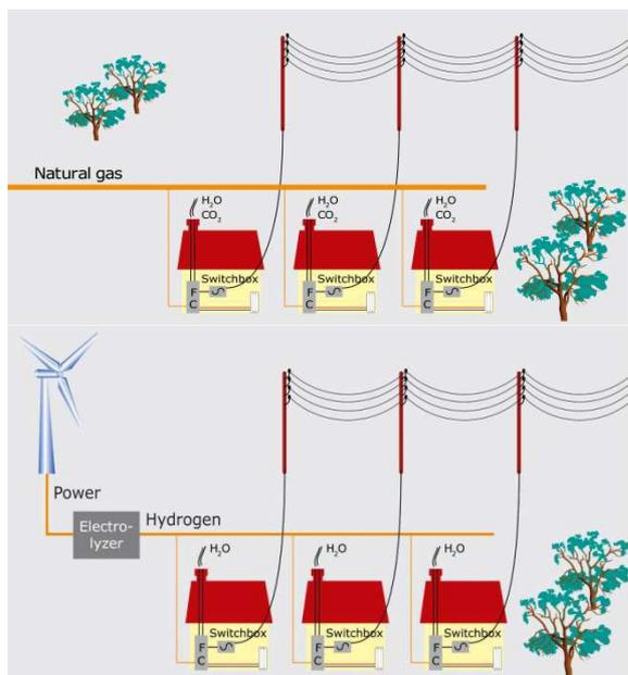
Figure 2: Two energy system designs for fuel cell operation.
