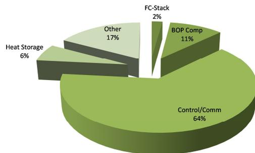
Figure 5: Fault statistics for hydrogen PEM units, phase 2.
