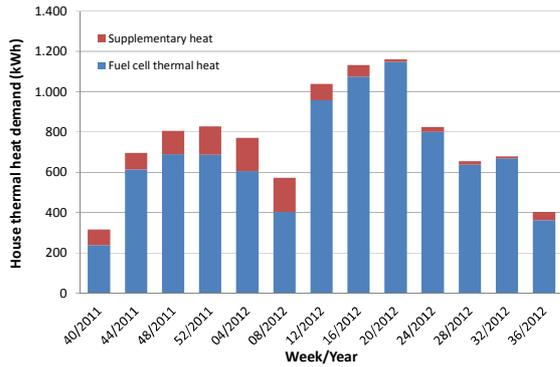
Figure 8: Thermal heat supply from a hydrogen PEM Gamma 1 fuel cell unit and supplementary heating (House 18).
