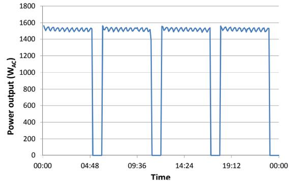
Figure 6: Operation pattern for a hydrogen fuel cell CHP unit in a simulated smart-grid situation (House 1).
