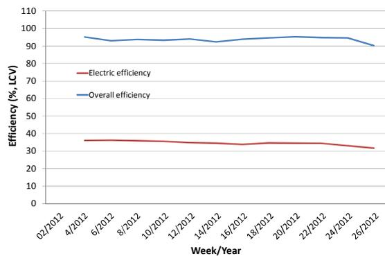
Figure 11: Electric and overall efficiency during 5 months for a field test of a natural gas PEM Beta unit (House 2).
