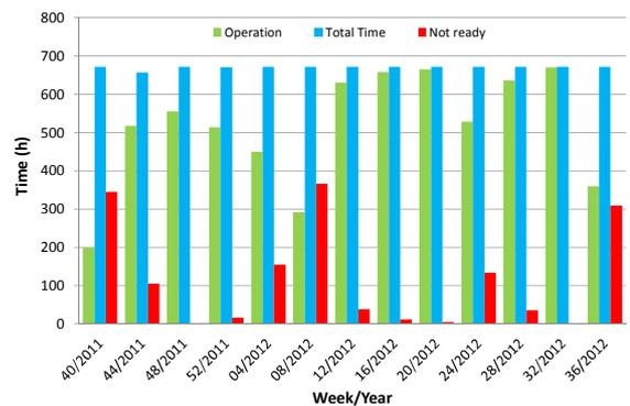
Figure 7: Operating example for a hydrogen PEM Gamma 1 fuel cell unit (House 18).
