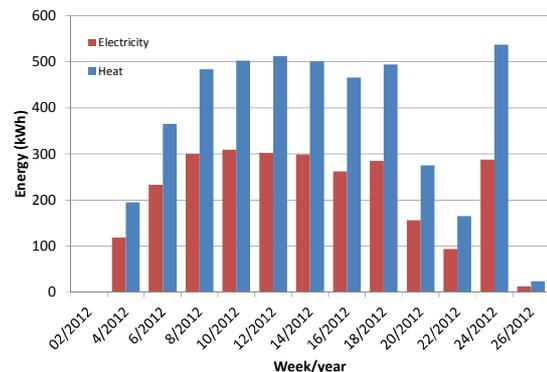
Figure 10: Operating conditions and performance for a selected natural gas PEM fuel cell during the first 5 months of operation (House 2).
