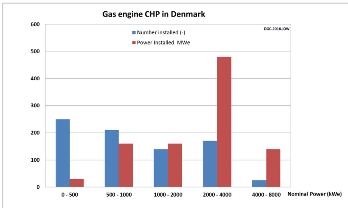
Figure 4 Overview of the gas engine population with regard to engine size, 2016 reference (nominal power, number of units and the total power for each power segments)
