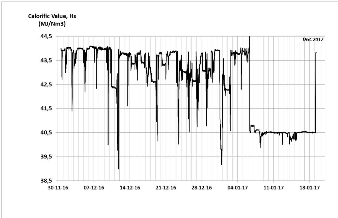
Figure 6 Example of measured gas quality at a CHP plant in the southern part of Jutland. The measurement was made during December/January 2016/2017.
