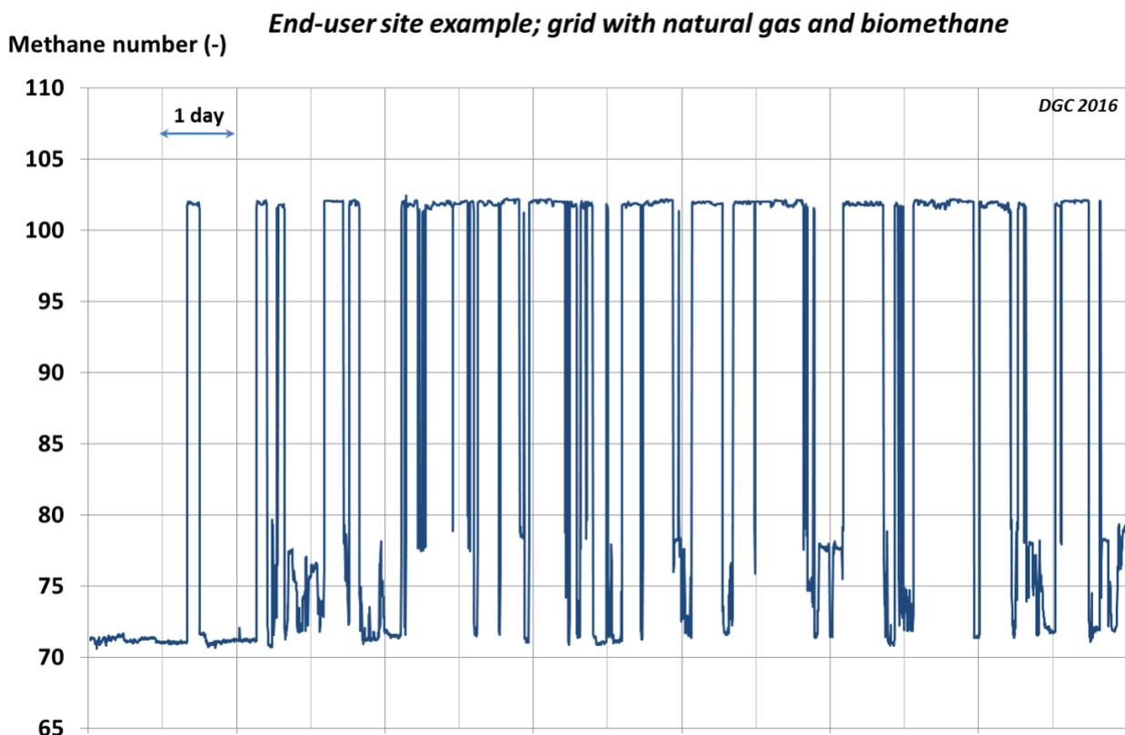
Figure 5 Example of gas quality (Methane Number) at a CHP plant in the central part of Denmark. The measurement was made early 2016.
