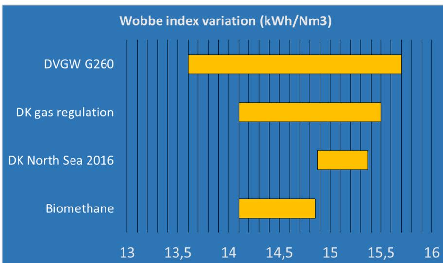
*Figure 3 The Wobbe Index acceptance range (DVGW and Danish regulation). And the actual range for gas supplied from the North Sea in 2016 and for upgraded biogas (bio-methane).*
