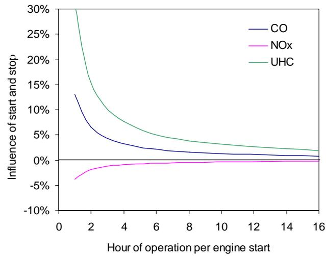
*Figure 2. The relative influence of start and stop on the emissions depending the operation time per engine start. Emissions are compared to steady state full load operation. Average value of examined pre-chamber engines.*
