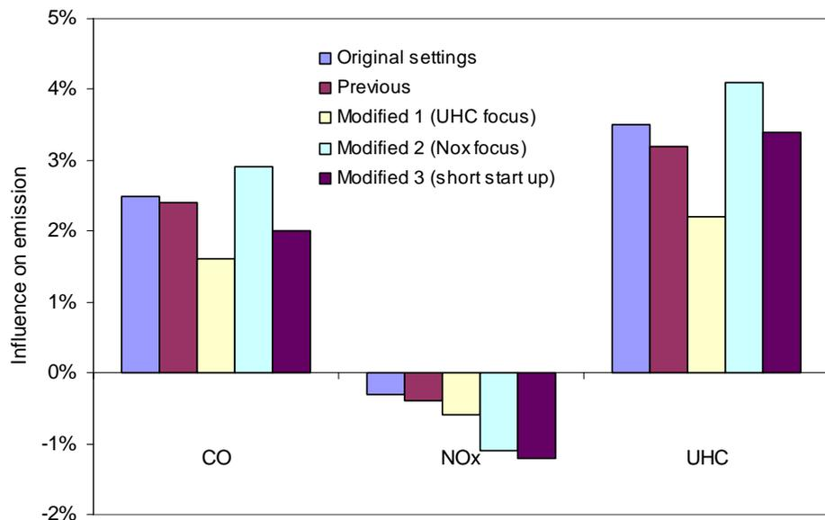
*Figure 3. The influence of start and stop on the overall emissions for engine unit #2. One warm start per 8 hour of operation compared to steady state full load operation.*
