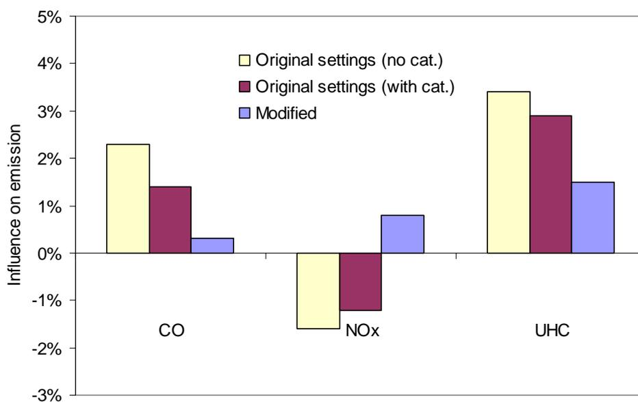
Figure 5. The influence of start and stop on the overall emissions for engine unit #4. One cold start per 8 hour of operation compared to steady state full load operation
