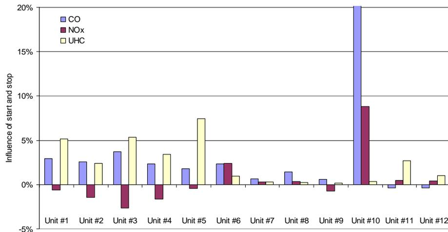
Figure 1. The relative influence of start and stop on the emissions from the examined units. One warm start per 8 hour of operation compared to steady state full load operation.
