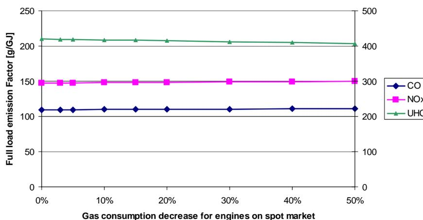
Figure 6. Sensitivity of reduced numbers of operation on full load emission factors for plants operating on the spot market.
