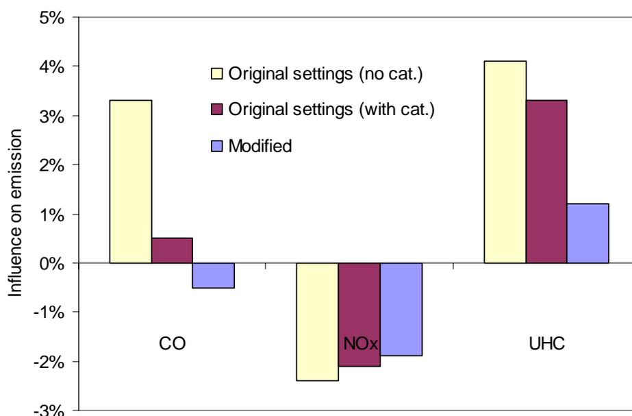
Figure 4. The influence of start and stop on the overall emissions for engine unit #4 . One warm start per 8 hour of operation compared to steady state full load operation.
