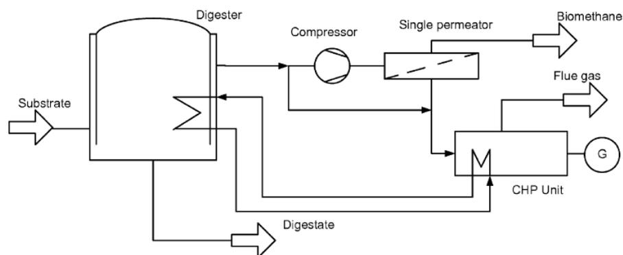
Figure 4. Simplified flowsheet for a single-stage configuration with CHP unit. From /18/.
