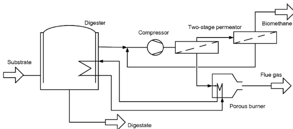
Figure 5. Simplified flowsheet for a two-stage configuration with permeate burner. From /18/.
