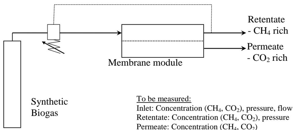
Figure A1. Sketch of the setup for membrane test.
