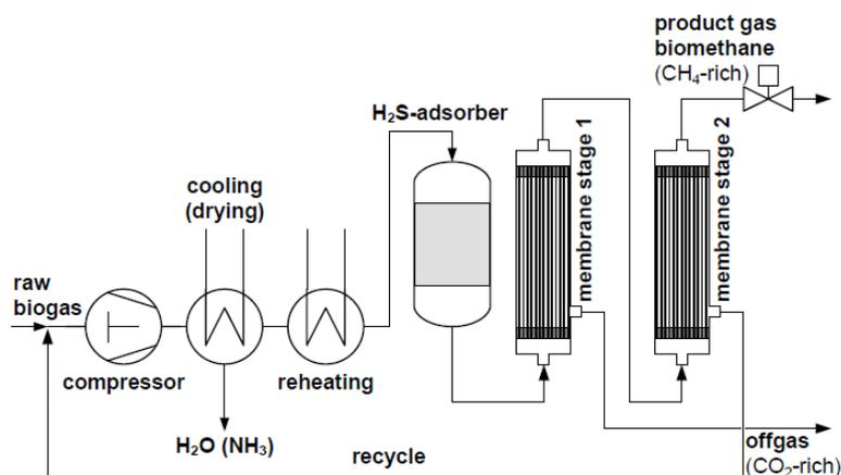
Figure 7. Flowsheet including the pretreatment before separation of the plant in Bruck/Leitha, Austria. The same unit as shown in Figure 5. From /16/.
